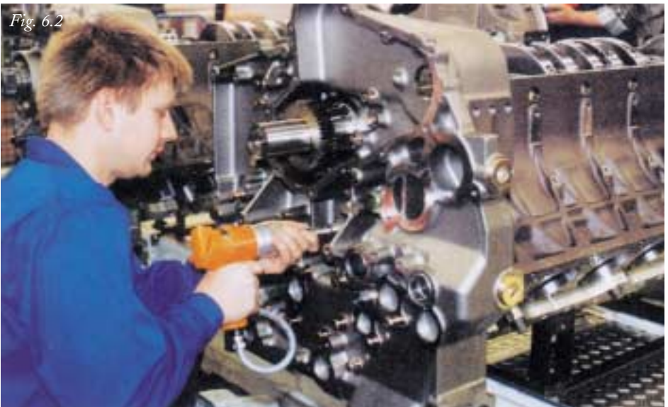
Fig. 6.2 illustrates a Cleco model #160PTH pulse tool being used to assemble a classic MTU engine. photo: Norbert Barlmeyer
